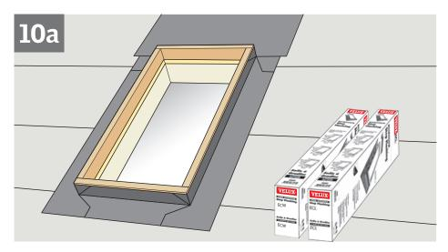
For thin roofing materials, use flashing ECL. ECL is designed for roof pitches 10°-60°.
