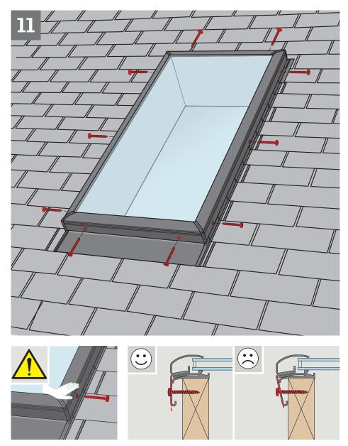
Centre the skylight on top of the curb and secure with 45 mm pan head stainless steel screws provided. Screws will penetrate the curb by at least 19 mm.
