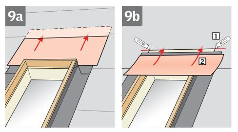
To allow for proper drainage, interweave felt with additional standard roofing underlayment as shown in 22 for new construction applications.
