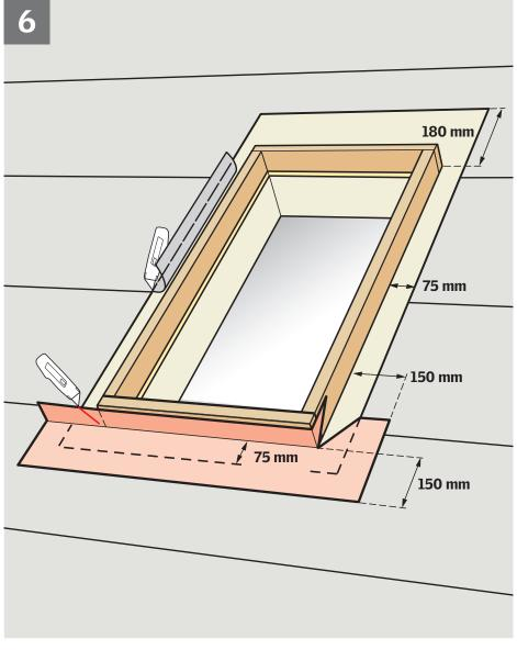
Skylight curbs should be completely wrapped in self-adhesive membrane to ensure waterproofing. To achieve this waterproofing, consider using VELUX adhesive skylight underlayment ZOZ 216 (225 mm wide).
