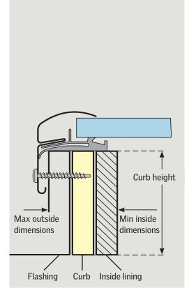
Build curb according to measurements in the chart. Curb height and attachment should comply with building codes and regulations and be secure enough to transfer the skylight loads to the framing members.
