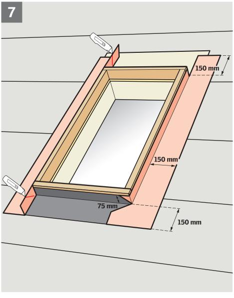
Consider wrapping the curb with VELUX adhesive skylight underlayment ZOZ 216 and create water-shedding laps over felt at bottom and sides of skylight 6, 7.
