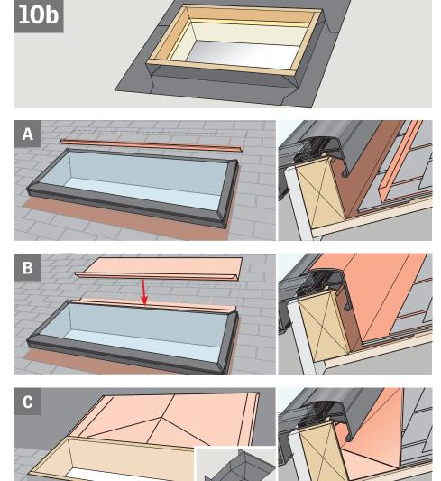
If custom-made flashing is used, consider options **A**, **B** or **C**.
